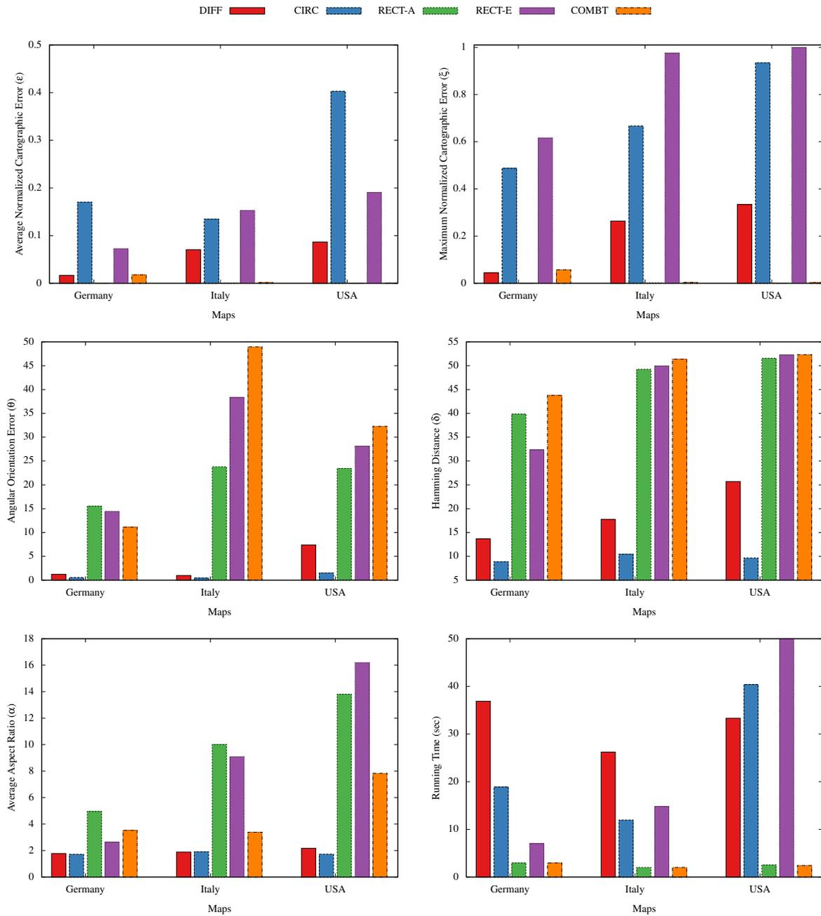
**Figure 7:** Average normalized cartographic error  $\epsilon$ , maximum normalized cartographic error  $\xi$ , angular orientation error  $\theta$ , Hamming distance  $\delta$ , average aspect ratio  $\alpha$  and running time for all algorithms (the iterative algorithm RECT-E was stopped after 50 seconds).
