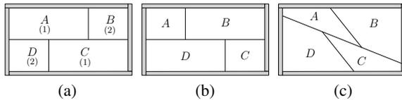
**Figure 2:** Three cartograms for a map with an area assignment for four states (A, B, C, D with desired areas 1, 2, 1, 2, respectively), containing (a) cartographic error, (b) topology error and (c) shape error. There is no cartogram with no cartographic error, topology error and shape error.
